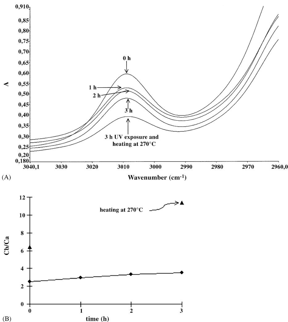
Fig. 8. (A) Spectra of corn oil samples exposed to ultraviolet radiation and heated. (B) The total amount of carbonyl compounds vs. UV exposure time.
