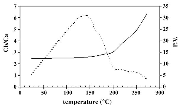
Fig. 7. Effect of different heating temperature on: (a) peroxide value (P.V.) (dashed line) and (b) the total amount of carbonyl compounds (solid line) (heating time was 30 min).
