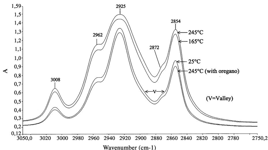
Fig. 5. Spectra of corn oil samples heated at 165 and 245 °C (with and without the addition of oregano) in comparison with the corn oil spectrum at room temperature.
