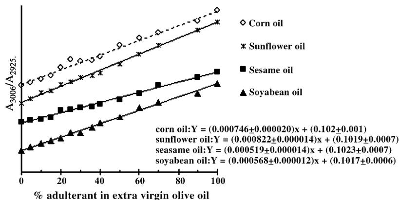
Fig. 4. Monitoring the adulteration of extra virgin olive oil with various vegetable oils with the use of the ratio  $A_{3006}/A_{2925}$ . Curves are arbitrarily offset.
