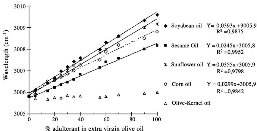
Fig. 3. The 3009  $\text{cm}^{-1}$  band shift vs. the percentage of adulterant (soyabean oil, sesame seed oil, sunflower oil, corn oil, olive-kernel oil) in extra virgin olive oil.
