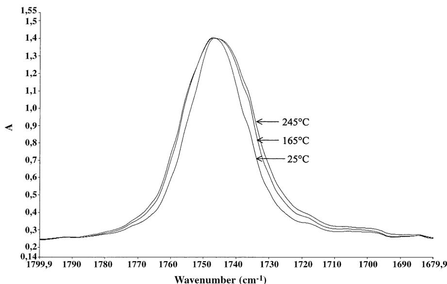
Fig. 6. Spectra of corn oil samples heated at 165 and 245 °C in comparison with the corn oil spectrum at room temperature.
