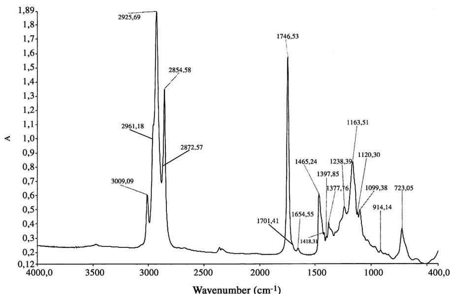
Fig. 1. FT-IR spectrum of a corn oil sample at room temperature (25 °C).
