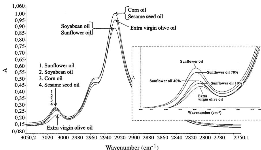
Fig. 2. Spectra of extra virgin olive oil and vegetable oils at 3050–2750  $\text{cm}^{-1}$ . In the inset spectra of extra virgin olive oil adulterated with sunflower oil at  $\sim 3006 \text{ cm}^{-1}$ .
